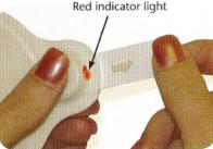
The red indicator light confirms that the device is operating properly. To avoid sleep disruption, the brightness of the red indicator light is minimized and is only visible in a dark location.
